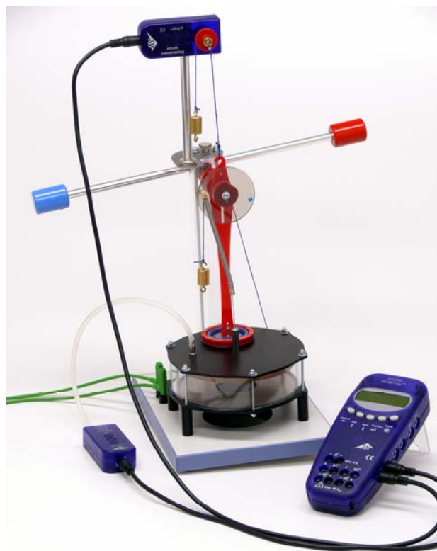
Fig. 9 Experiment set-up for recording a pV diagram
