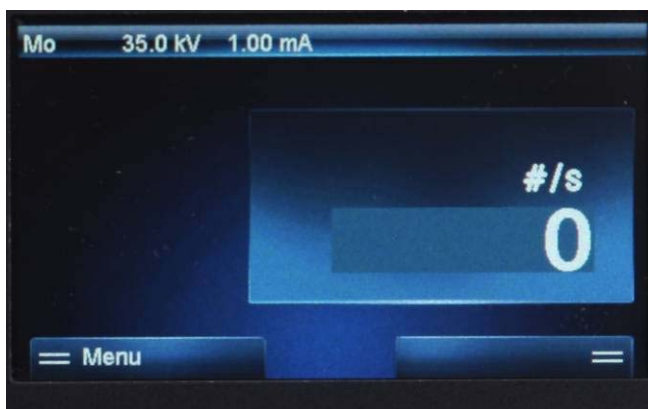
Fig. 10: Screen for controlling the unit at the front of the unit. The x-radiation is not activated.
