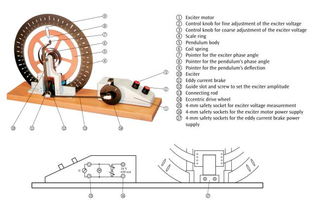
The torsion pendulum may be used to investigate free, forced and chaotic oscillations with various degrees of damping.
