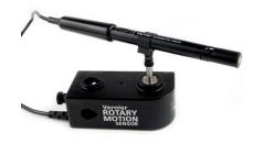
The thumb screw can be threaded into the back of the sensor allowing the Rotary Motion Sensor to be attached to a ring stand.
