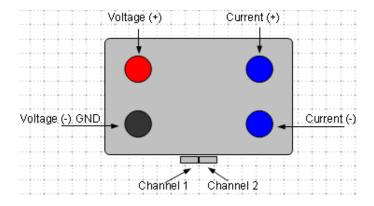
The probe has 4 safety type sockets for connection to the experiment and 2 telephone type sockets (RJ45) for connection to the interface (LabQuest/LabPro).
