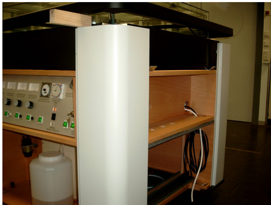
Figure 2.4: Side view of the cloud chamber with removed side walls. On the right hand side the feed through hole for the power cables can be seen. On the left hand side the operation panel (top) and the 2-Propanol storage vessel (bottom) are shown.
