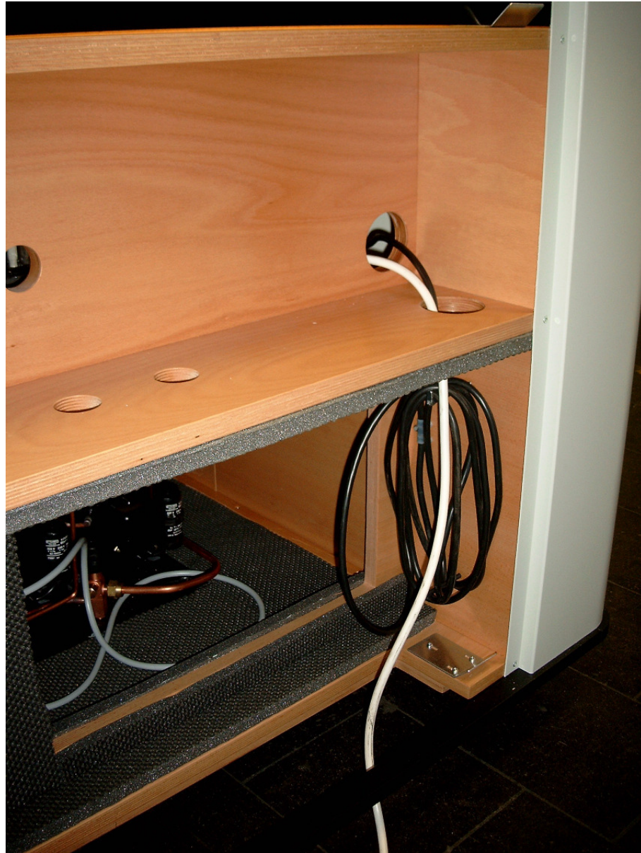
Figure 2.8: Feed through hole for the power cables. The black cable is the 230 V AC cable of the cloud chamber and the white cable is the supply cable from the grid – for the USA this means 115 V AC.
