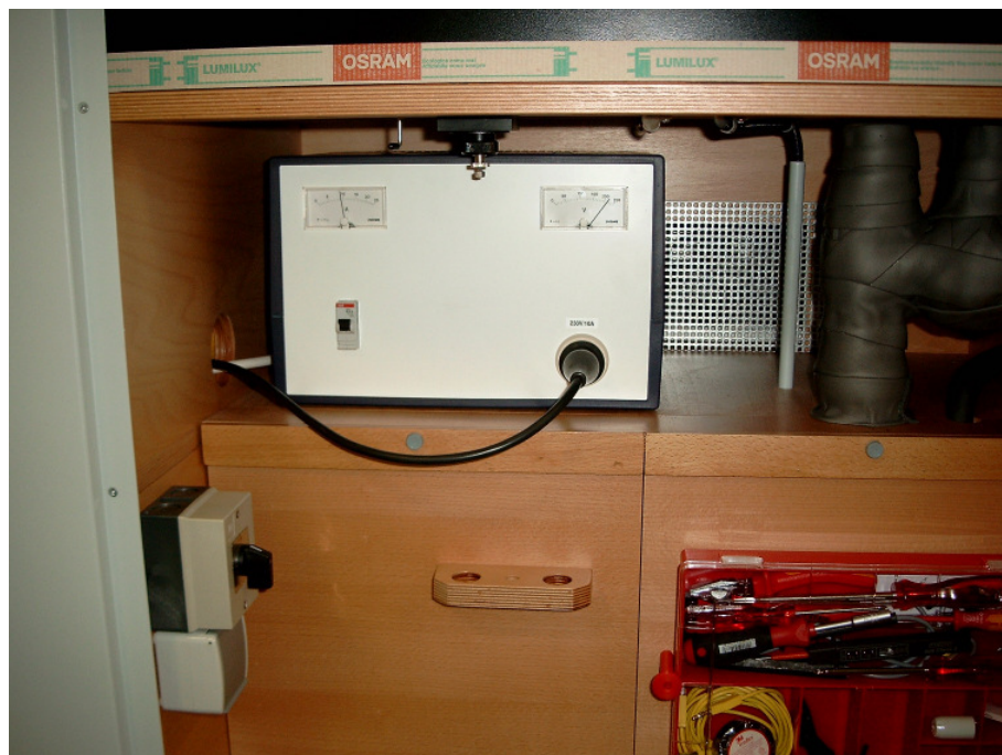
Figure 2.10: Inside view of the PHYWE cloud chamber PJ 80/3 09043.93 with installed PHYWE transformer XX330461, installed feed through dummy insert and plugged in 230 V AC plug in the socket of the PHYWE transformer XX330461.
