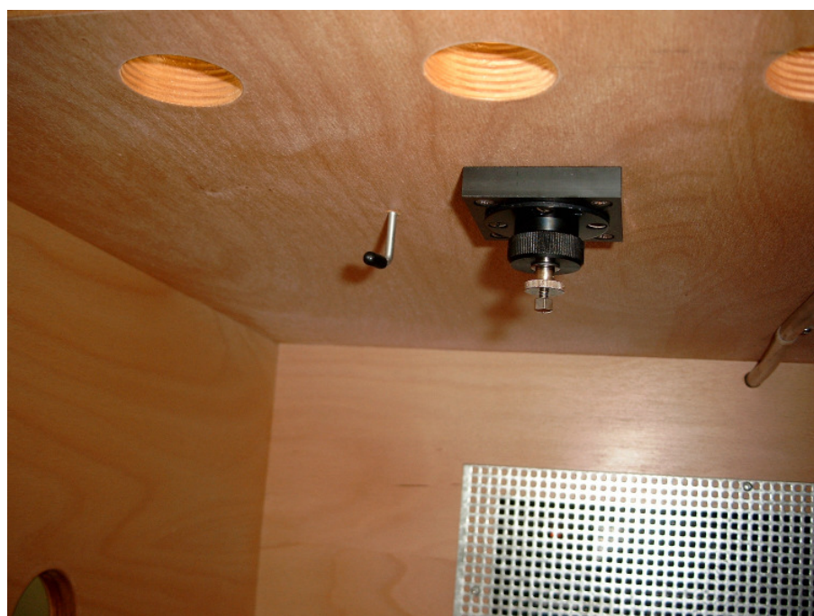
Figure 2.5: Inside view of the cloud chamber showing the feed through for radioactive sources – a dummy insert is installed.
