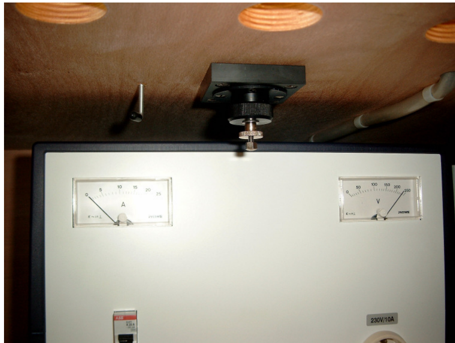
Figure 2.9: Inside view of the cloud chamber with installed PHYWE transformer XX330461 and feed through dummy insert.
