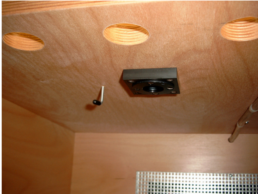
Figure 2.6: Feed through for radioactive sources with removed dummy insert. The insert has to be removed for the installation of the PHYWE transformer XX330461 inside the base of the cloud chamber.
