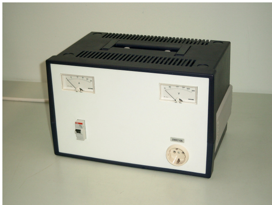
Figure 2.1: Front side view of the PHYWE 100...200 V AC/230 V AC transformer XX330461. This transformer has an input voltage of 100...200 V AC and an output voltage of 230 V AC. The total power provided by this transformer is 2 kVA. The two analogue displays show the current (A) and voltage (V) of the output. On the left hand front side of the front panel a 25 A safety overload switch. On the right hand front side a 230 V AC socket with ground contacts (shock proof plug/socket) is installed. In this socket the plug of the diffusion cloud chamber (black cable) has to be installed.
