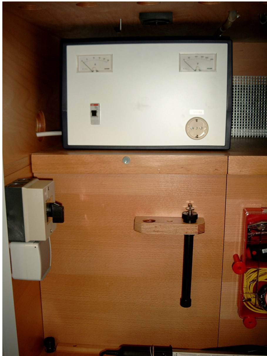
Figure 2.7: Inside view of the PHYWE cloud chamber PJ 80/3 with installed PHYWE transformer XX330461. The feed through dummy insert is stored into the wooden holder below the place of the transformer.
